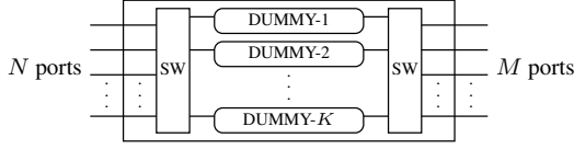
Figure 1. An N:M switch with at most K concurrent connections may be modeled by two full crossbar switches and K dummy resources.
