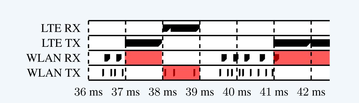
WLAN RX desensitized by LTE TX; WLAN TX prevented by LTE RX
