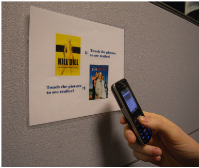
Figure 2. Physical Interaction of Device and RF Memory Tag
